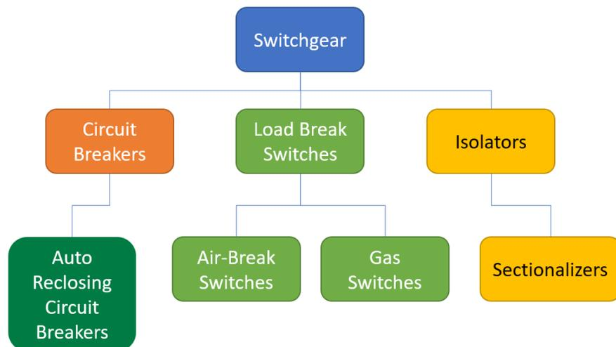
Figure 1: Simplified Switchgear Classification
