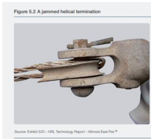
The major fire event at Kilmore South in Victoria was started by a SWER overhead line cable which had been dislodged from its saddle. When the cable eventually broke and landed on the grounded cable stay, the old Oil filled Hydraulic Recloser that was operating on this line did not have a modern controller or remote communications, meaning that it was left to Reclose and reenergise the line. It is highly
