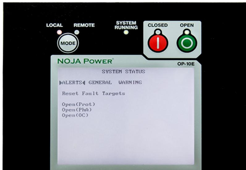
Close Up of the NOJA Power RC Controller HMI Interface Panel
