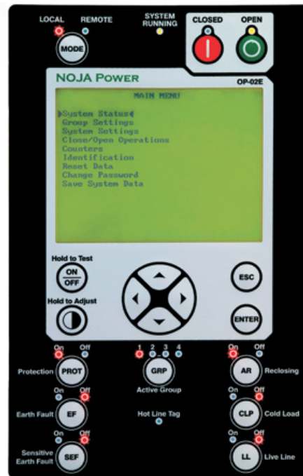
Local Control Panel
