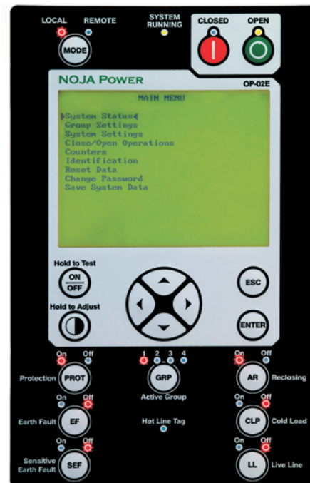
Local Control Panel
